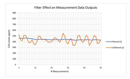
The graph above shows the effects of the filter on the  $CO_2$  measurement data (Z or z). The unfiltered output is shown in orange and the filtered output shown in blue.
