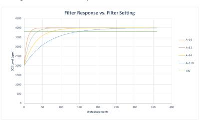
The graph above shows the effect of the filter on response times. Increasing the filter setting increases the measurement output response time.  $T_{90}$  is the time to 90% of reading. The SprintIR<sup>®</sup>-6S takes 20 readings per second. The flow rate was set at 0.2I/min.
